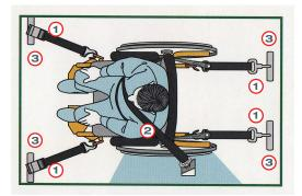
1 WHEELCHAIR RESTRAINTS 2 OCCUPANT SECUREMENTS 3 FLOOR ANCHORAGES
